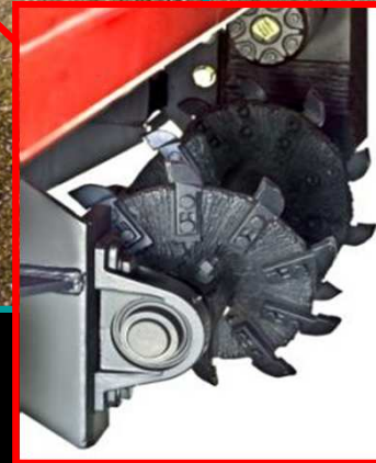
Rotary Auger distributes recycled material into windrow
